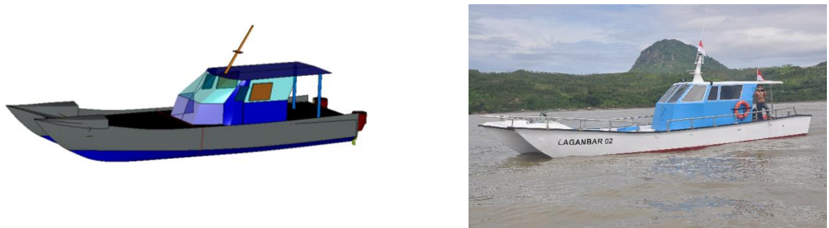
Figure 4. Catamaran 3-D view -MAXSURF (left) and sea trial of laganbar (right).
