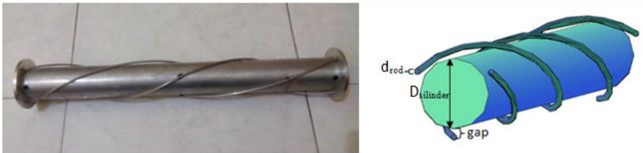
Figure 1. The model cylinder covered by triple helical rods with gap and the nomenclature.
